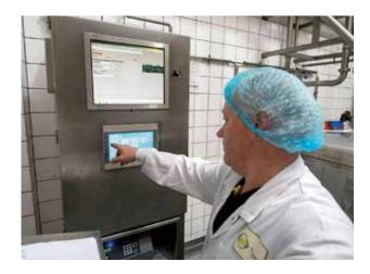
Once the packaging is used in production, the pallet barcode must be scanned to update the stock position and register the time of processing to maintain traceability.
